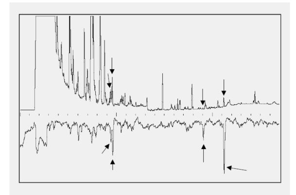
Figure 3. Coupled GC-electroantennogram of volatiles from virgin female box elder bugs. Top, GC detector response, expanded to show trace components; bottom, inverted trace, simultaneous response recorded from the antenna of a male bug. The 4 small to trace components that elicited consistent strong responses from the male antenna are indicated by arrows. The first two and the 4<sup>th</sup> have been identified, whereas the 3<sup>rd</sup> component is not yet known.
